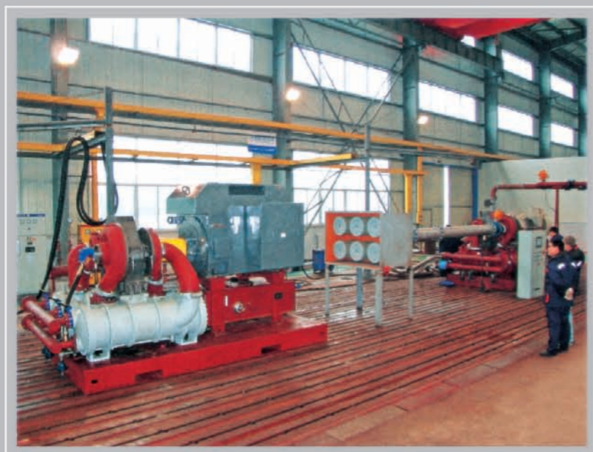
压缩机运转试验台 Compressor Operating Test Stand
